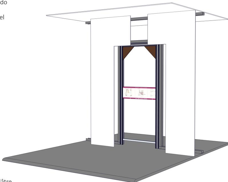
**5** Cut the plasterboard sheets avoiding that there aren't any joints at the upper corners of the doorframe
